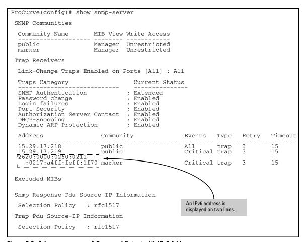
Figure 5-8. "show snmp-server" Command Output with IPv6 Address
